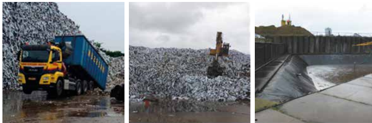
Picture 5 Examples of storage bin (left), solid base storage (mid), and drain water collection (right)
