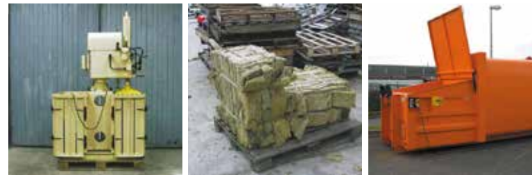
Picture 4 Example of baler (left), baled slabs without plastic (mid), and press container (right)
