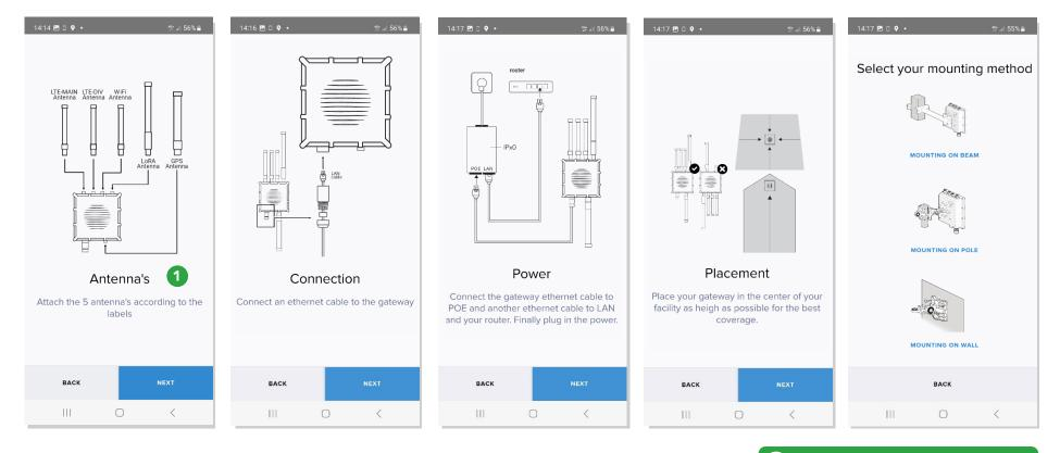
Connect the antenna. NOTE: 2 antennas are delivered with the gateway. Ideally, use the longest antenna.
