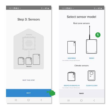
) Select the sensor to install and follow the onscreen instructions. Additional details on GroSens sensor installation, please refer to the GroSens installation manual
